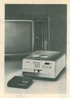
Toshiba linear video recorder achieves tape speed of 6 m/s and a playing time of an hour with 220 tracks on continuous loop.
