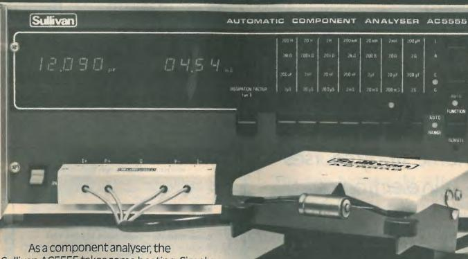
Sullivan AC5555 takes some beating. Simply slot the component into the jig and watch the equipment select the correct range and function and provide a read-out of the correct value...automatically. It's as simple as that.
